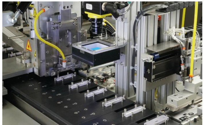
The Kinematic Automation Matrix 2390 with dedicated MHS cutting and placing technology at 60 ppm in this configuration.
