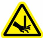
**SHEAR CUT HAZARD:** The interlocked Lexan blade guard and is designed to prevent access to the blade during operation.
