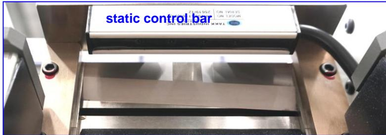
A static control bar is provided to de-ionize strips after they have passed through the blade set. The static control power supply is located inside the machine and is active when the machine is on. The static control bar is attached to a steel rail mounted at the rear of the unit. The groove in the static control bar should be cleaned with clean dry pressurized air on a regular basis. See Section 7.2.
