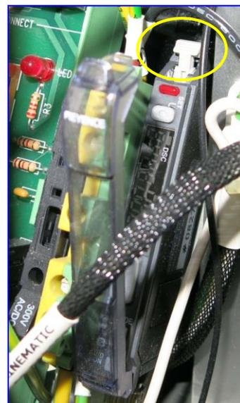
**Do not over-tighten the lock screw or setscrew. Fiberoptic cable is easily damaged.**
