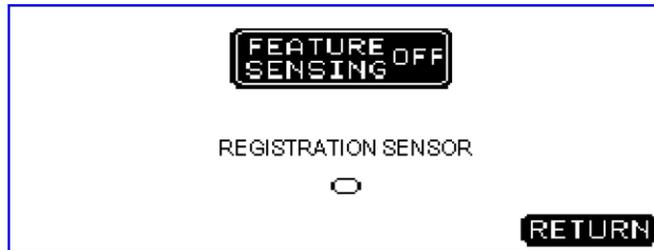
The **FEATURE SENSING ON/OFF** button is used to enable or disable the optional feature registration. When Feature Sensing is ON, the signal from the sensor amplifier will be used each cycle to control the pinch drive and locate the material correctly before the shear is activated.
