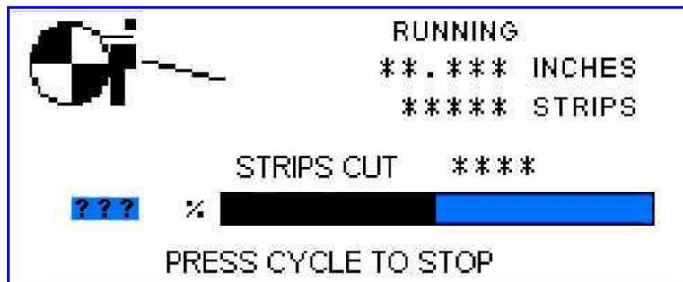
It also shows the number of strips to be cut, the strip size (in inches or millimeters) the actual number of strips already cut in this batch, and a bar graph, which shows the progress (as a percentage) of the run.
