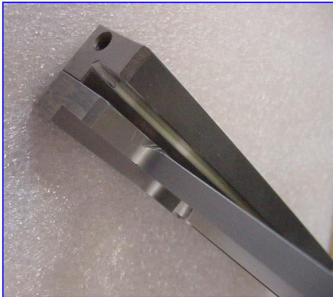
Grease in the Die Block Groove
