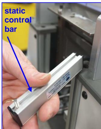
7. Pull the static control bar up until the entire cable has been pulled through the gap in the top plate. **check image for new switch**
