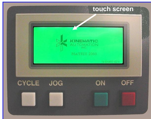
**CYCLE** – Starts the process of cutting the programmed number of strips. (If pressed during a batch run it halts that run and resets the strip counter.)
